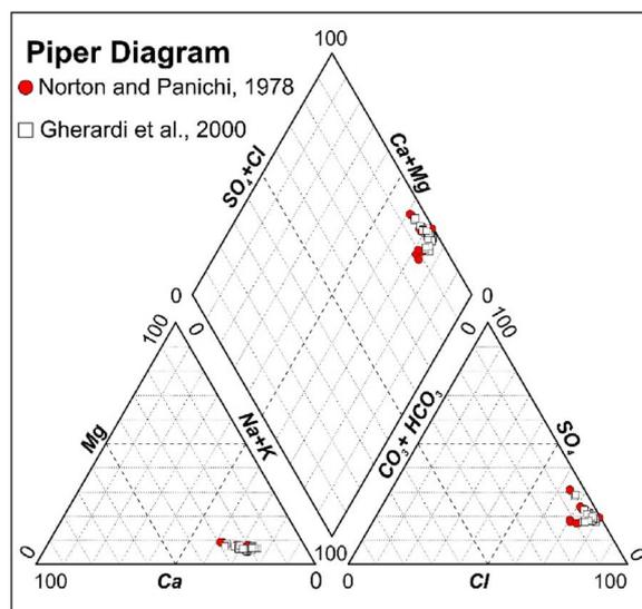
Fig. 2. Piper diagram of the chemical analyses on the Euganean thermal water (circle: Norton and Panichi, 1978; square: Gherardi et al., 2000) suggesting that the facies of the water is sodium-chloride.
