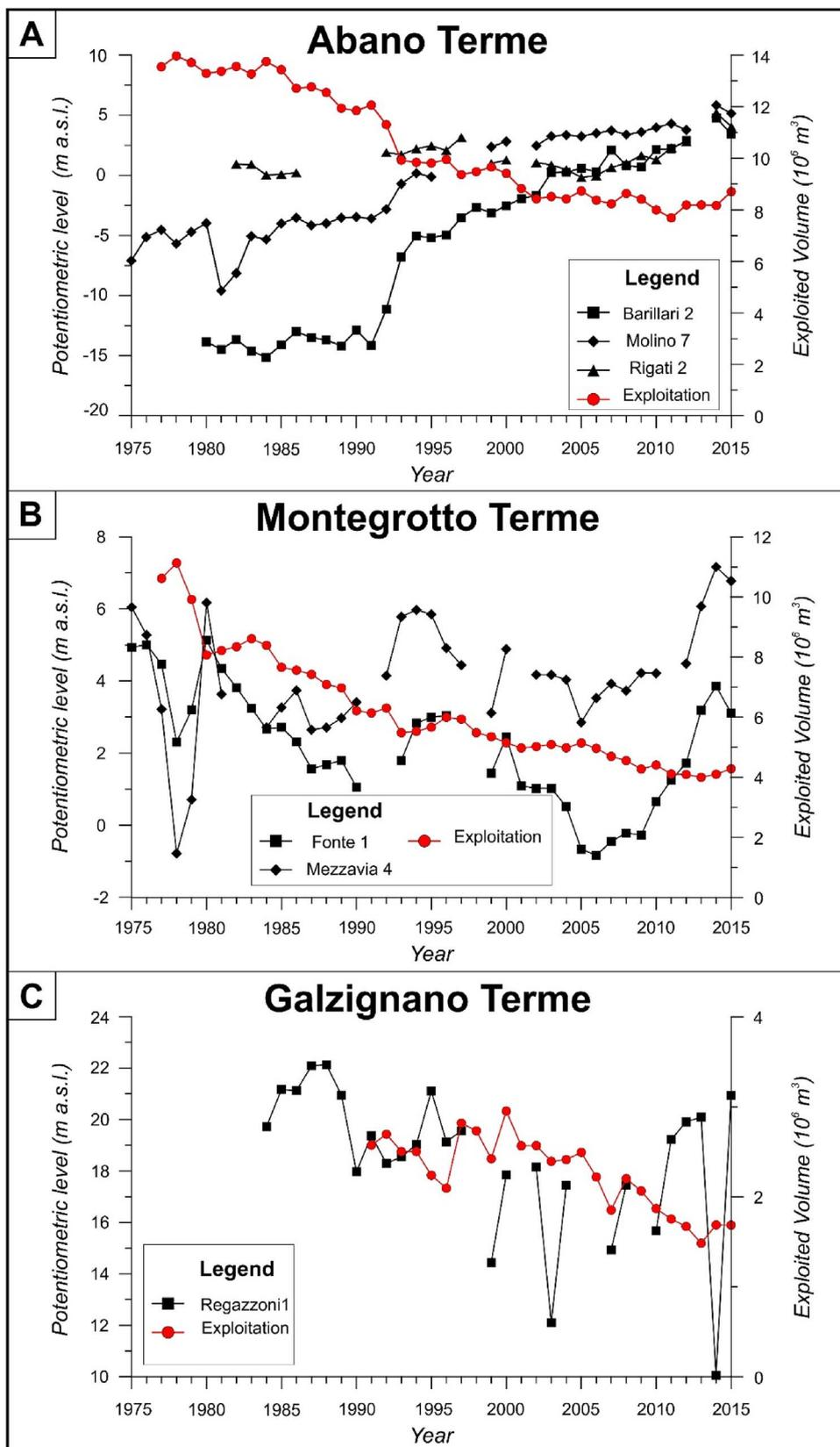
Fig. 6. Annual mean potentiometric level measured in the wells of the monitoring network since 1975 (Table 1; Fig. 3). The time series are grouped for the different areas of the EGF (A: Abano Terme; B: Montegrotto Terme; C: Battaglia Terme and Galzignano Terme), and they are compared with the total annual extracted water volume.
