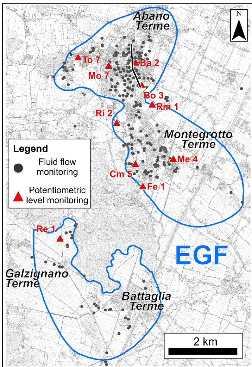
Fig. 3. Distribution of wells equipped with flow meters (gray dots) or used for the continuous monitoring of the potentiometric level (red triangles; see Table 1 for the acronyms). The main towns of the EGF are also reported.
