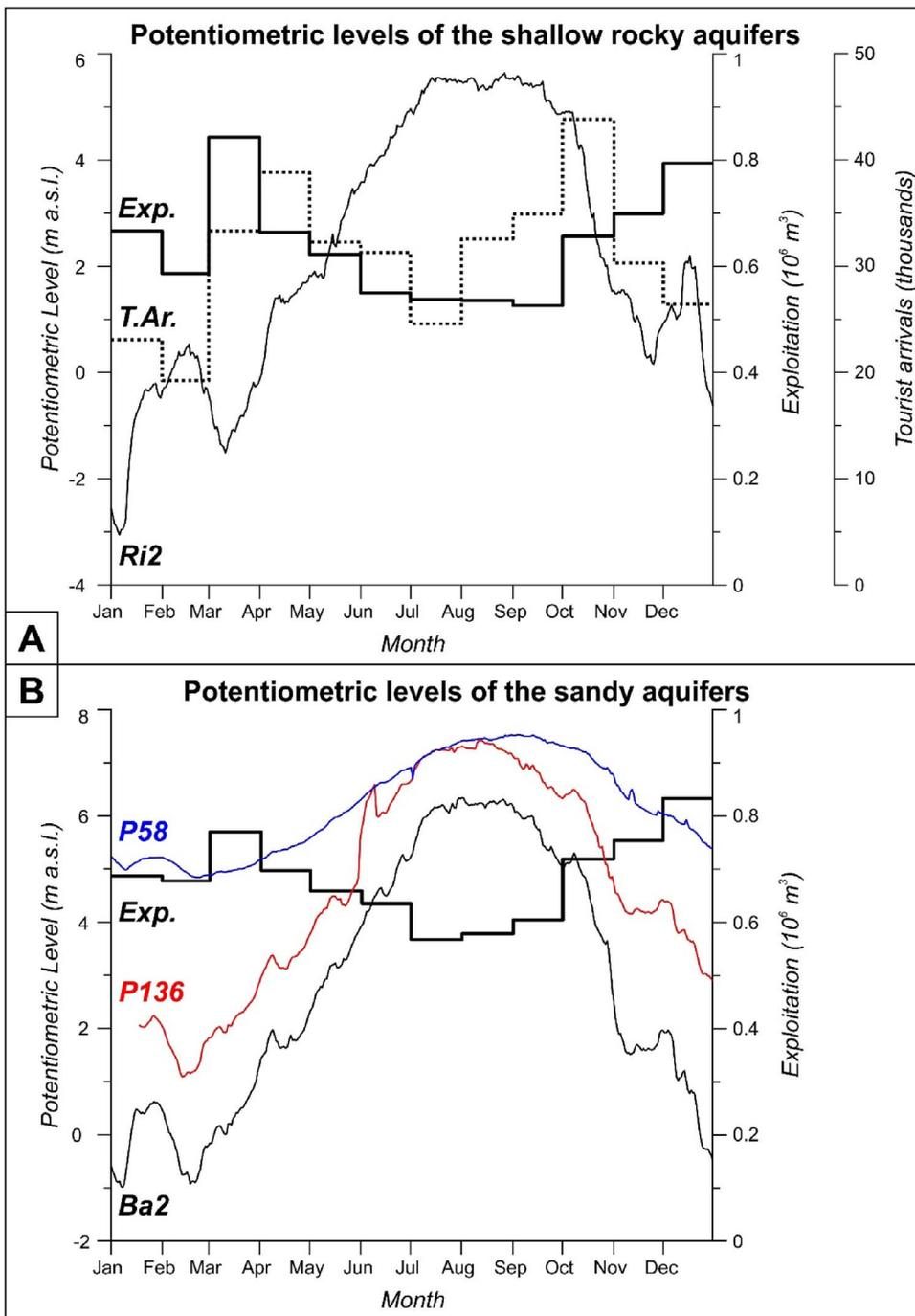
Fig. 4. Annual trends of the potentiometric level in the thermal aquifers of the EGF (A: year 2011; B: year 2012). The trend is comparable in both the 300–600 m deep rocky aquifers (Ri2 in A and Ba2 in B) and the shallow sandy aquifers of the alluvial cover (P58 and P136 in B). The observed seasonal variations can be associated with different exploitations (Exp.) and in turn to the different rates of incoming tourists (T.Ar.).
